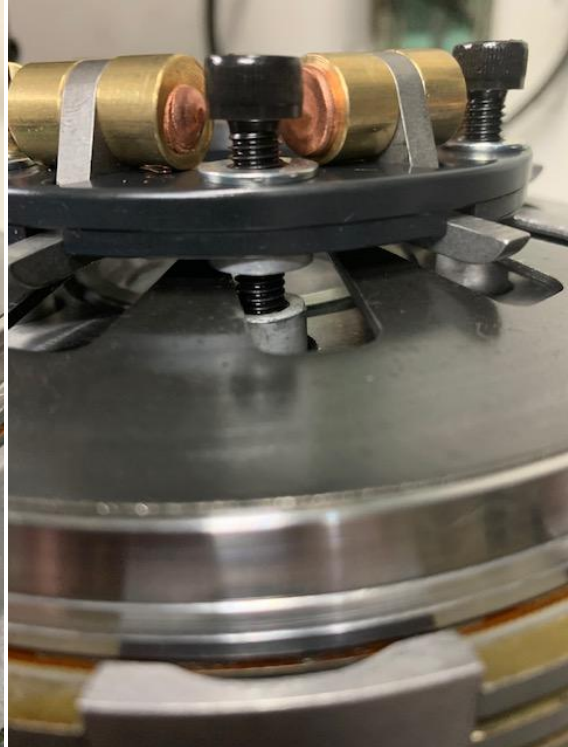
Pic.10 Incorrect Diaphragm is not aligned to hub boss.
